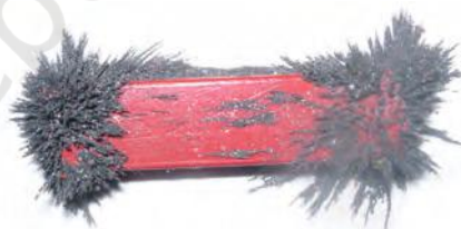
Fig. 10.7 Iron filings sticking to a bar magnet
